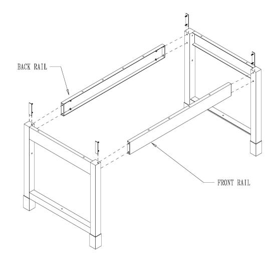
1) ASSEMBLE 4" FRONT AND BACK RAILS USING STUD
